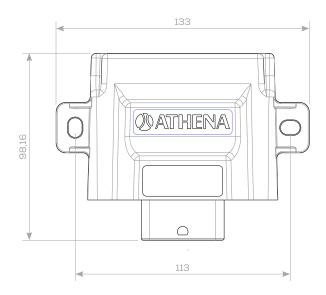
S-SERIES is the engine control units' family, developed by Athena's electronic division for the complete management of the EFI engines. This platform is extremely flexible and subjected to strict validation tests, based on Automotive standards.
